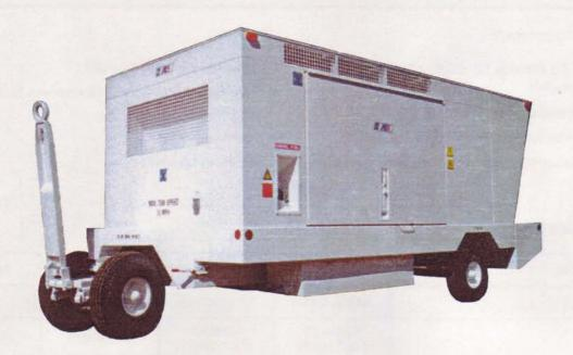
The 600 Series are truck or trailer mounted continuous flow jet engine starting units producing 180 PPM at up to 40 psig start air pressure.
